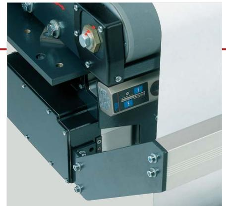
Infra-red sensor FR 50 on a rotary offset press
