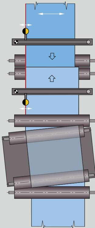
**Web to web guiding by the web center line with two support beams**
