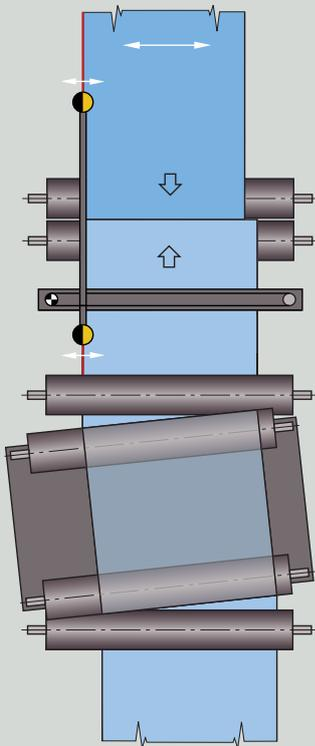
**Web to web guiding by the web edge with two support beams**
