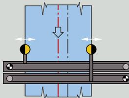
Guiding by the web center which does not correspond to the machine center with motor-driven sensor positioning for both sides (Automatic edge search)
