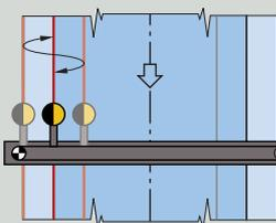
For larger oscillating strokes, the mechanical sensor set point is change via motor
