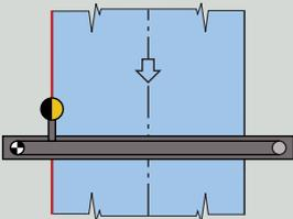
This basic version features a carriage and a drive unit in order to position the sensor at the required position.
