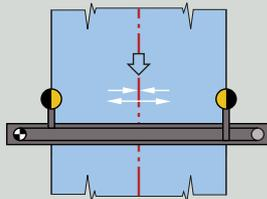
This version comprises two carriages, linked to one another via a toothed belt. The former are protracted or extended together via a drive unit.
