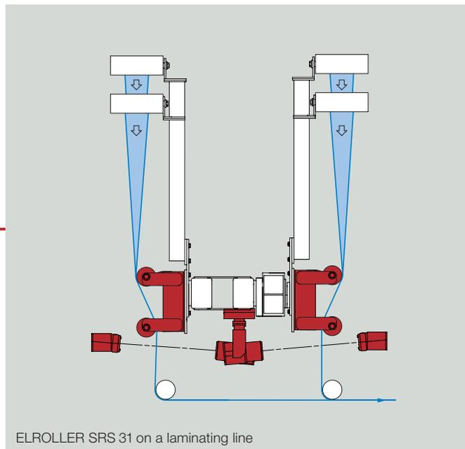
ELROLLER SRS 31 on a laminating line
