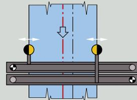
This support beam also features two carriages, each with its own independent drive unit. This means that the left and right sensors may be adjusted independently of one another. Due to a synchronous drive control, web offsetting is thus possible across the full width of the web.
