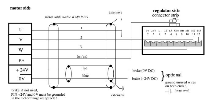
Motor-line-shield: on both ends, extensively connected!
