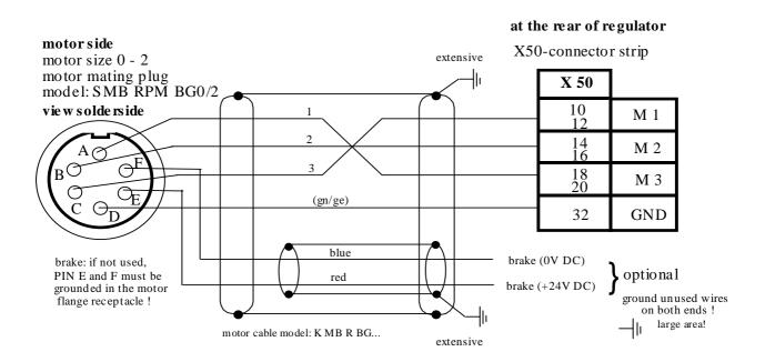
Motor-line-shield:on both ends, extensively connected!
