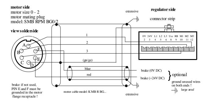
Motor-line-shield:on both ends, extensively connected!
