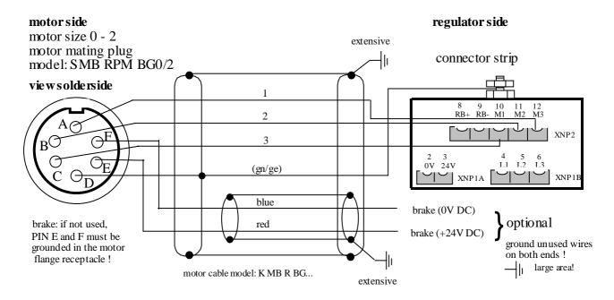
Motor-line-shield:on both ends, extensively connected!
