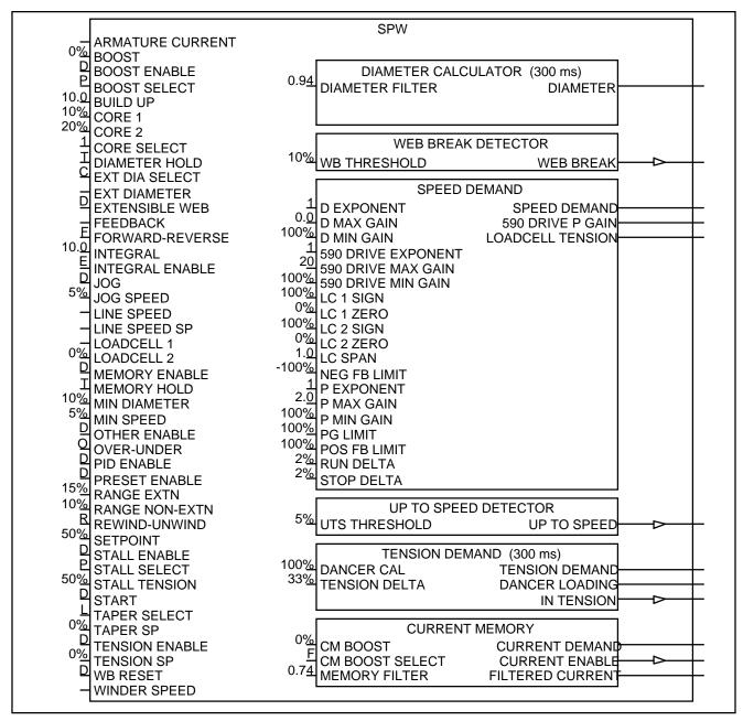
This function block is made up of five sub-function blocks: "Diameter Calculator & Web Break Detector", "Up to Speed Detector", "Tension Demand", "Speed Demand", and "Current Memory". Each of these are described below. Unless otherwise noted, all parameters are persistent, can be preset, and have set and get methods. All logic
