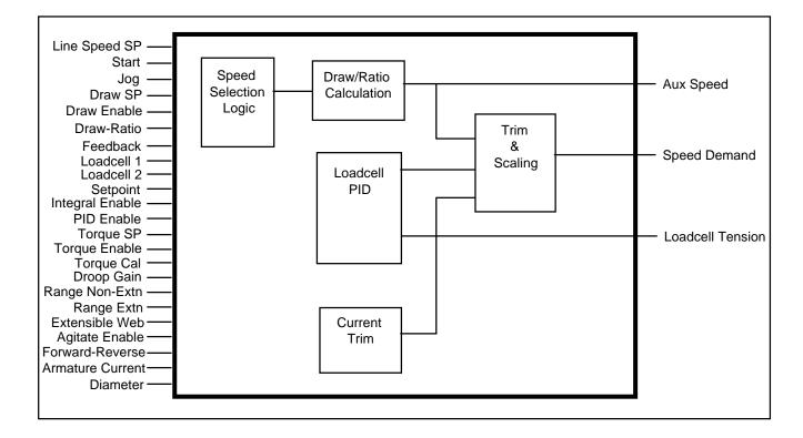
This function block is made up of five sub-function blocks: "Speed Selection Logic", "Draw/Ratio Calculation", "Trim & Scaling", "Loadcell PID", and "Current Trim". See the *Line Drive/Loadcell PID* data sheet (RG354173) for a description of the Loadcell PID. The other blocks are described below. Unless otherwise noted, all parameters are persistent, can be preset, and have set and get methods.
