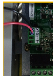
5V can be supplied by USB using the 1002-00-00 CLONE MODULE
