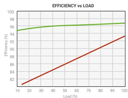
■ XMV660 MV Drive    ■ PWM GTO current source inverter
